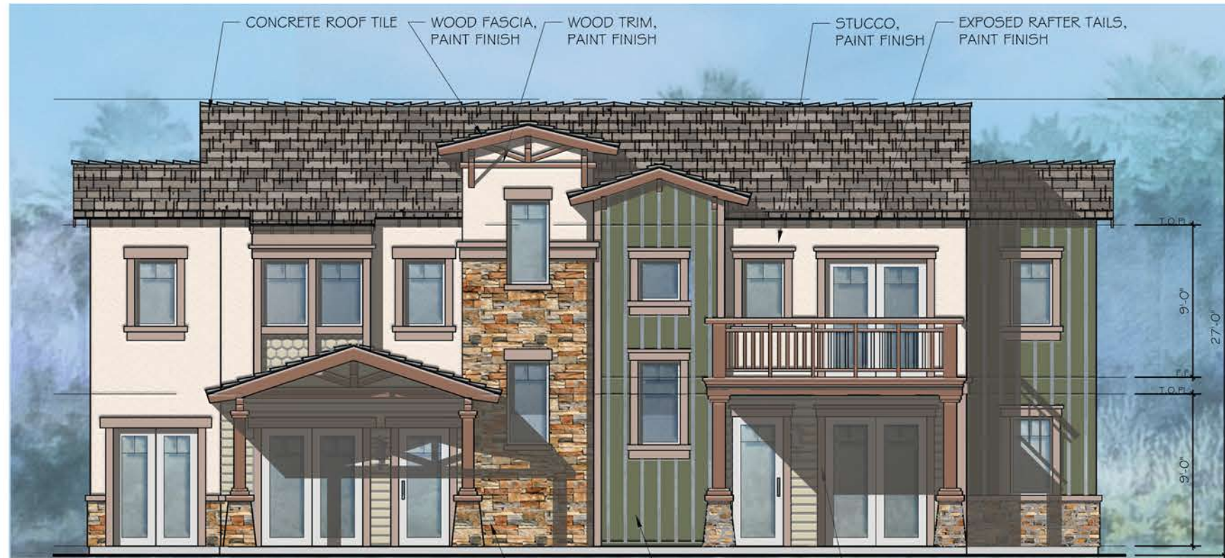
STONE VENEER HARDI PANEL SIDING, PAINT FINISH WOOD TRIM, PAINT FINISH WEST ELEVATION SCALE: 1/4"=1'-0
