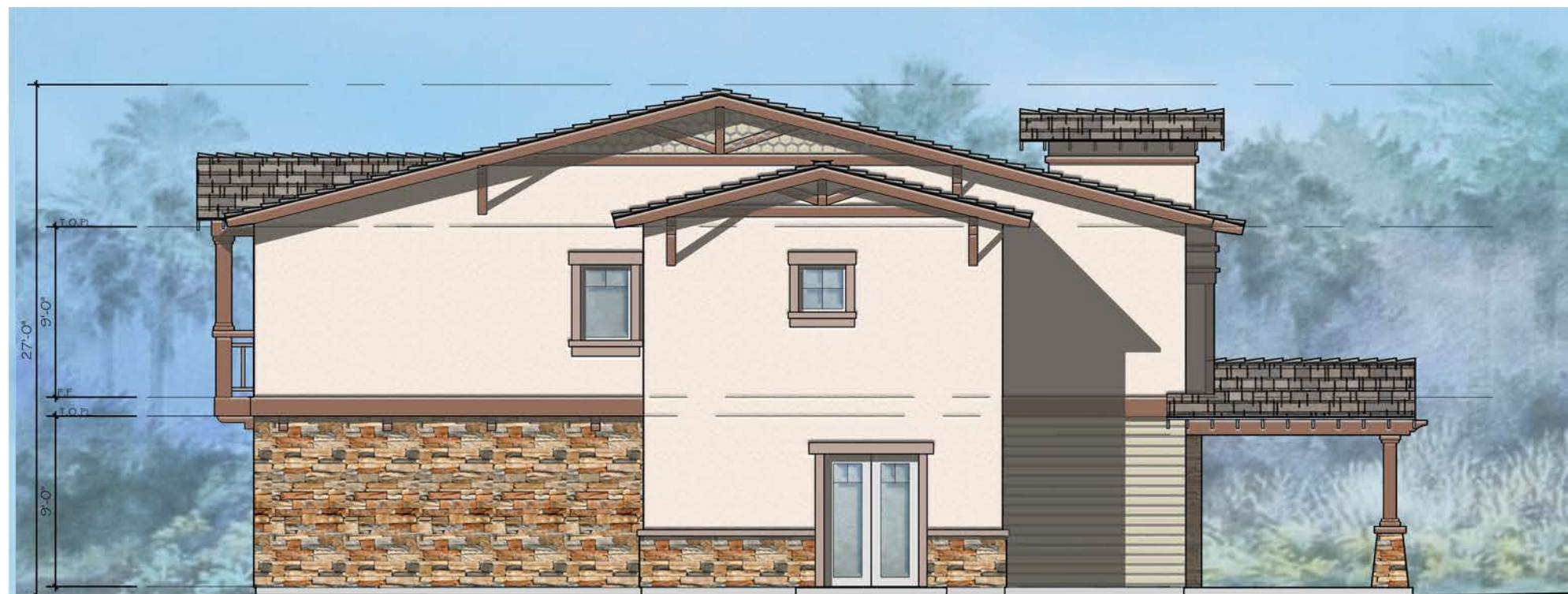
STONE VENEER HARDI PANEL SIDING, PAINT FINISH WOOD TRIM, PAINT FINISH WEST ELEVATION SCALE: 1/4"=1'-0
