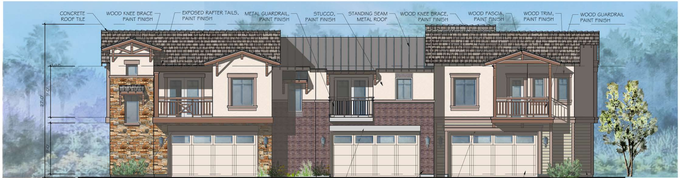
WOOD LINTEL, PAINT FINISH DECORATIVE LIGHT FIXTURE CONCRETE LINTEL BRICK VENEER WOOD LINTEL, PAINT FINISH METAL GARAGE DOOR, PAINT FINISH HARDI PANEL SIDING, PAINT FINISH WEST ELEVATION SCALE: 1/4"=1'-0
