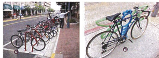
Bicycle parking can take many forms. A simple bike rack can be placed near the entrance of a storefront (a). Bike storage facilities can be more dynamic and enhance the brand or identity of an area, shown in (b) as part of a small parking lot. As new development occurs, there may be sufficient demand to set aside an on-street parking space exclusively for bicycle (c). Enhanced bike racks are a functional way of introducing public art into the streetscape (d).
